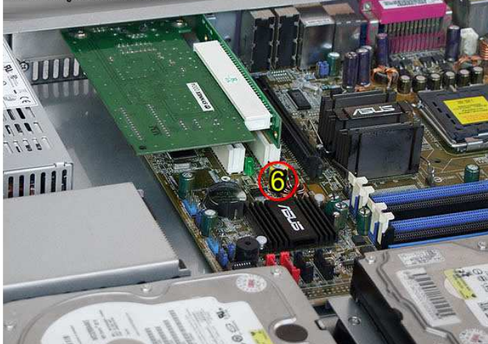
PCI 32bit riser card 6th slot position on MB
