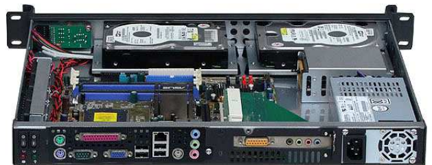
PCI-Express 16X riser card with extender 7th slot position on MB
