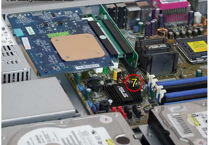
PCI-Express 16X riser card with extender 7th slot position on MB
